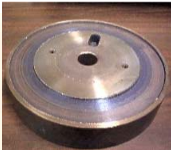
Figure 4. IBD wear on cast iron after FAST testing for 9 hours.
