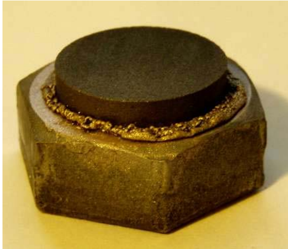
Figure 1. Vacuum Cu-Sil braze between IBD and carbon steel bolt head.
