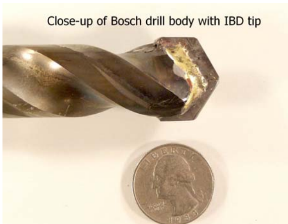
Figure 3. Standard bronze wire braze used to attach IBD tip to steel drill bit body.
